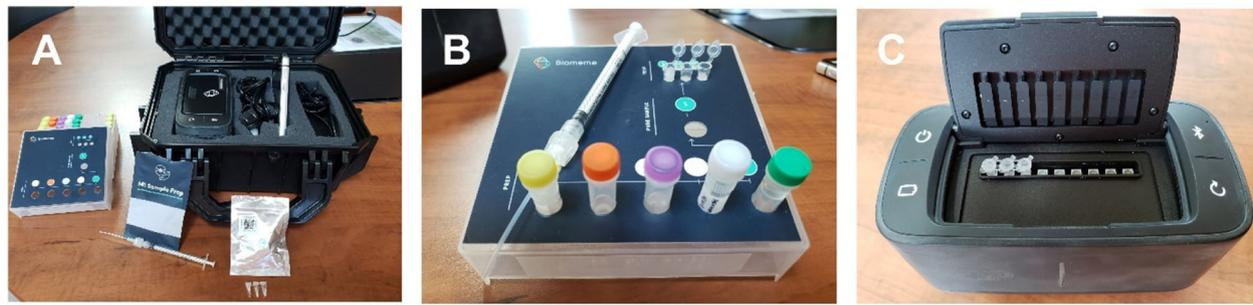
**Fig. 3** Overview of the Biomeme system. **a** complete set-up with PCR cyclometer and extraction kit. **b** Biomeme M1 syringe-based sample prep kit. **c** Biomeme battery operated mobile thermocycler
